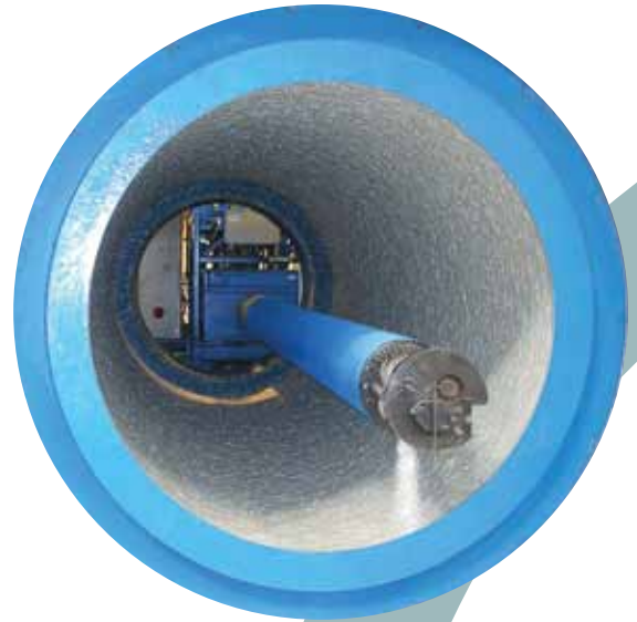
Centrifugal casting process patented by HOBAS
